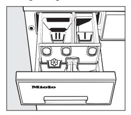
= Compartment soak/pre-wash. This compartment is also used for starch formulations when starching separately.
